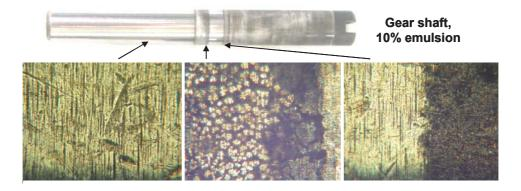
Fig. 10 Shaft gear surface after pump test
