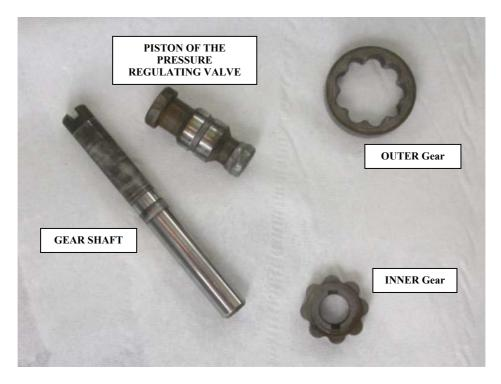
Fig. 8 Pump components under investigation
