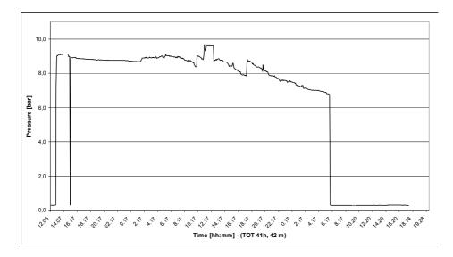
Fig.7 Pressure at pump outlet during the PO-LFO pump test
