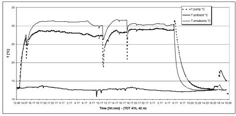
Fig.6 Temperatures during the PO-LFO pump test
