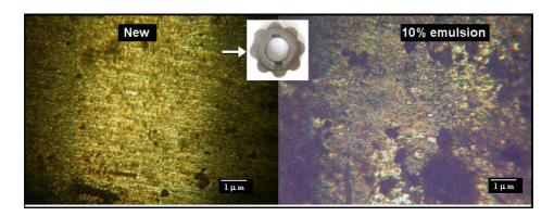
Fig. 9 Cog surface after pump test
